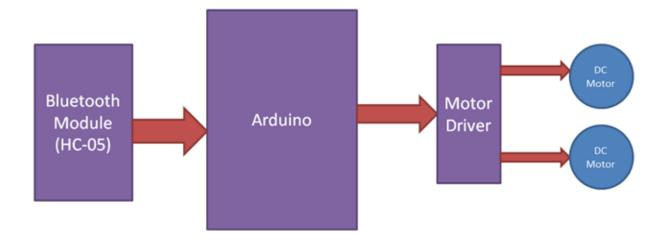
Bluetooth controlled car moves according to button touched in the android Bluetooth mobile app. To run this project first we need to download Bluetooth app form Google play store. We can use any Bluetooth app that supporting or can send data. Here are some apps' name that might work correctly.
